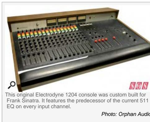
This original Electrodyne 1204 console was custom built for Frank Sinatra. It features the predecessor of the current 511 EQ on every input channel.
