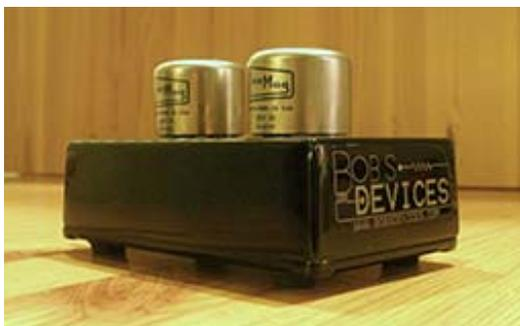
Over the past several weeks, I have had the pleasure of experimenting with Bob's Devices Cinemag Sky 30, a step-up transformer (SUT) used to passively raise the signal of low-output moving coil (MC) cartridges to the point where they can be amplified by a moving magnet (MM) phono stage. I will tip my hand early here: the Sky 30 SUT is a great
