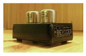
Over the past several weeks, I have had the pleasure of experimenting with Bob's Devices Cinemag Sky 30, a step-up transformer (SUT) used to passively raise the signal of low-output moving coil (MC) cartridges to the point where they can be amplified by a moving magnet (MM) phono stage. I will tip my hand early here: the Sky 30 SUT is a great
