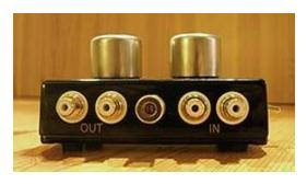
Bob Sattin, the owner-operator of Bob's Devices, hand-builds each of these devices and maintains meticulous quality control to ensure that the construction of each unit is of the highest standard. On his website, Sattin points out that internal connections are "resistance soldered using the American Beauty system which avoids heat damage to the delicate insulation on the hair-like wires of the transformers." In a
