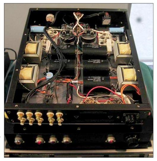
"In the case of the 6C33C-B, the tube is biased for a plate resistance of about 90 ohms. With a small amount of global feedback, the source output resistance will drop to about 12
