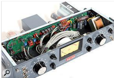
Inside the unit, it's mostly point-to-point wiring (with plug-in connectors).
