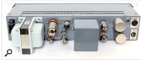
The rear panel hosts all the valves and transformers.
