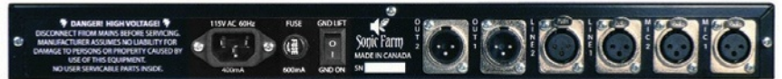
Figure 2: Creamer Plus' rear panel sports connections for mic inputs and line I/O.
