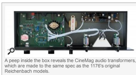
A peep inside the box reveals the CineMag audio transformers, which are made to the same spec as the 1176's original Reichenbach models.
